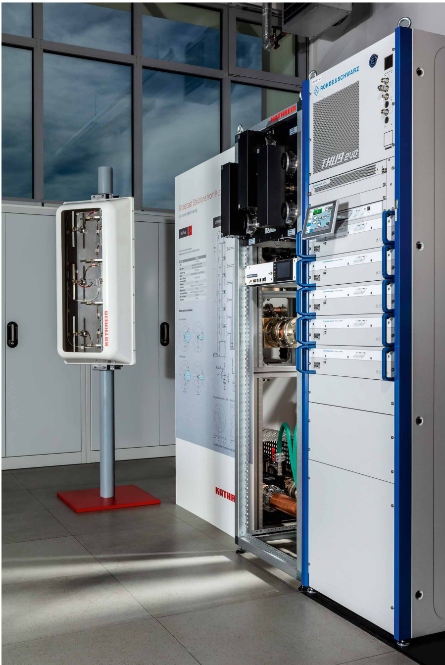
Fig. 2: The setup needed to transmit FeMBMS signals is not that complex. The test installation in the Ismaning station consists of the Rohde & Schwarz transmitter with a modified modulator and antenna equipment from Kathrein. On the left is an open version of the diversity antenna.
