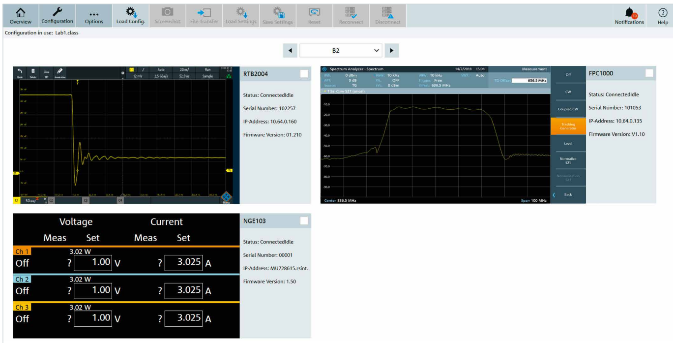
Fig. 3: The teacher can select each individual test instrument, capture the screen content and make settings.
