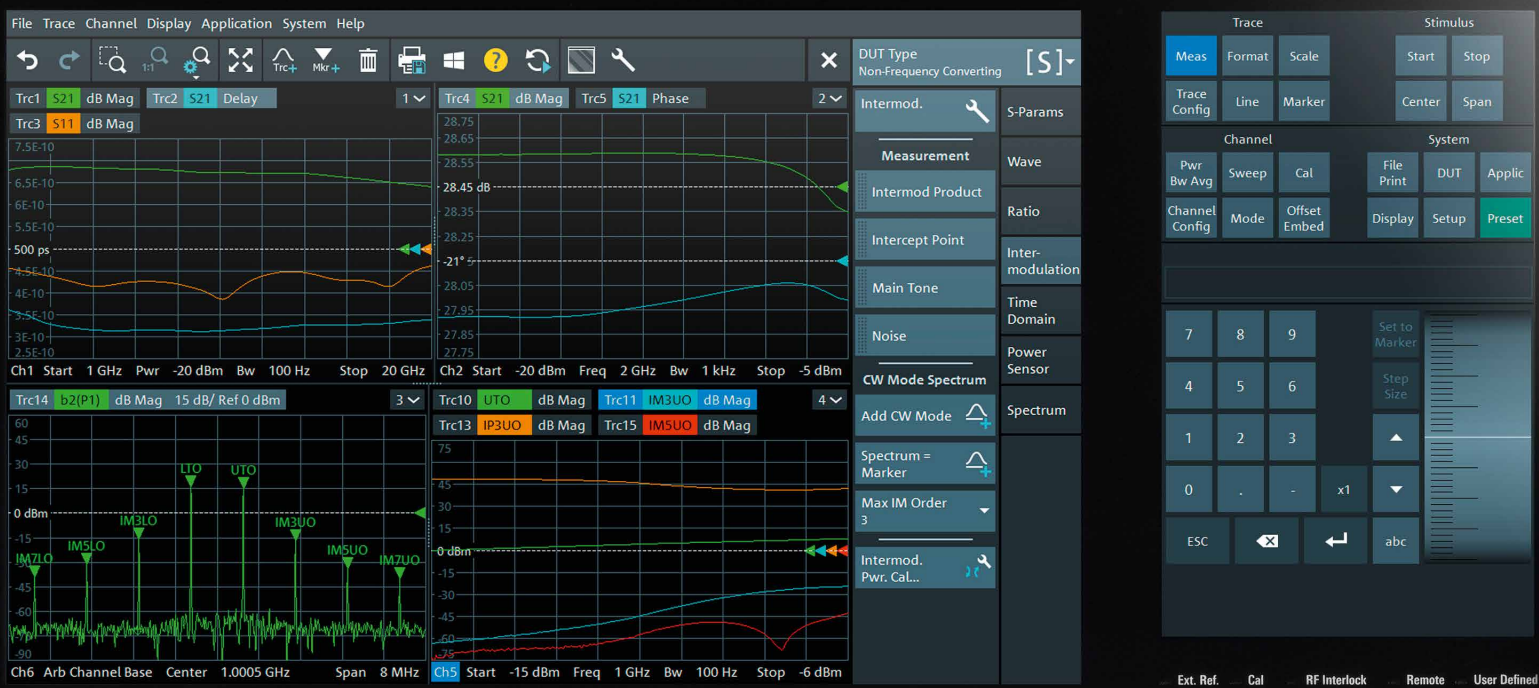
Fig. 2: The R&S®ZNA does not have any mechanical keys. All measurement-related data and menus are displayed on a large touchscreen. A smaller screen is used for general instrument configuration.
