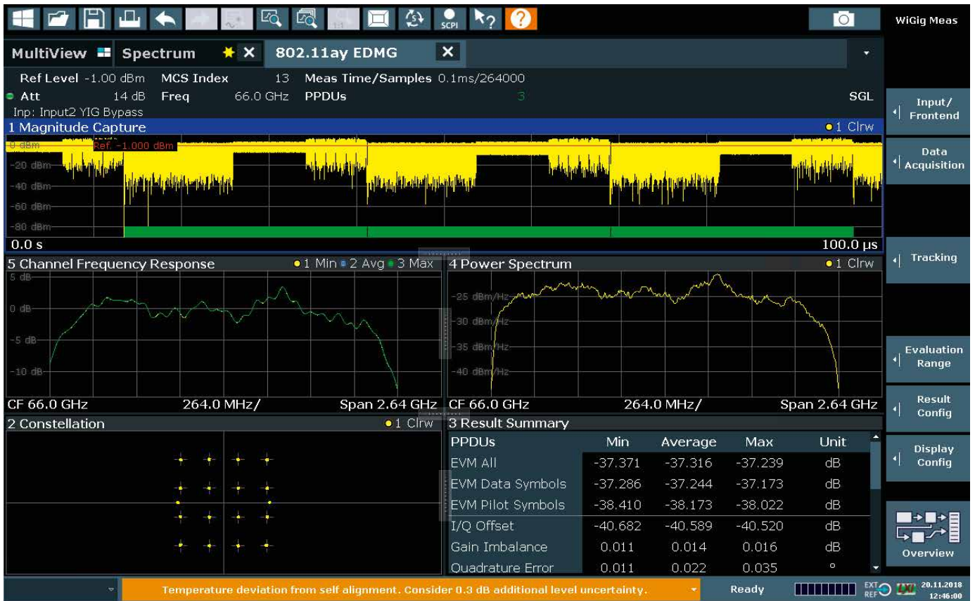
Fig. 2: Analysis of a 2 GHz wide WLAN 802.11ay signal. Along with graphical representation of the signal in the time and frequency domain, display of the constellation diagram and other results, users especially appreciate EVM and other numerical results.
