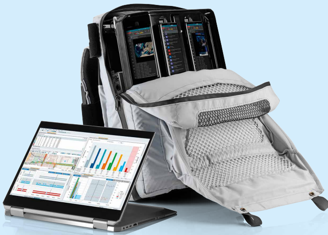
Fig. 1: The backpack has room for all required components. The Freerider4 is operated using a notebook or tablet.
