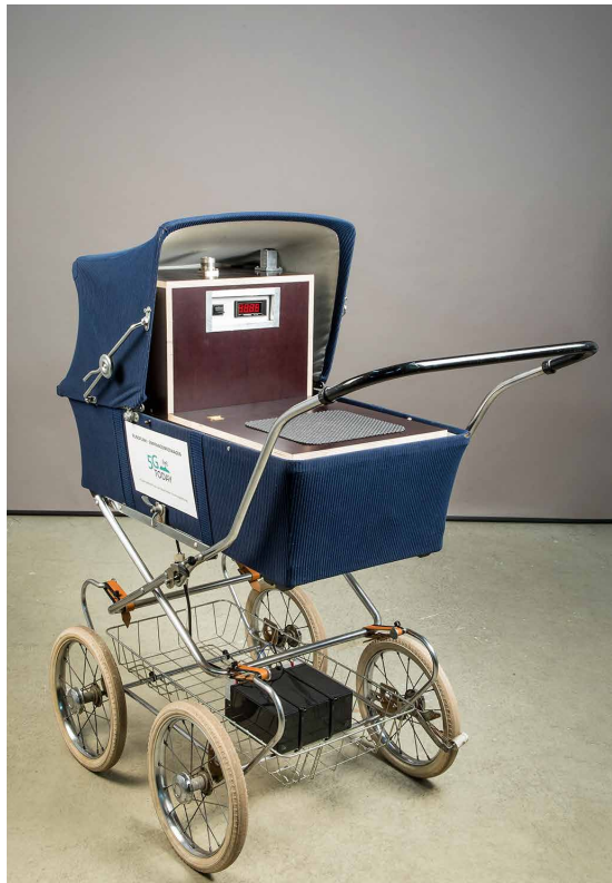
Fig. 3: The Kathrein measurement baby carriage (in transport mode on the left and in measurement mode on the right) combines retro charm with advanced analysis technology. It houses GPS and measurement antennas, an R&S®TSMW network scanner, a computer with signal analysis software and the power supply.
